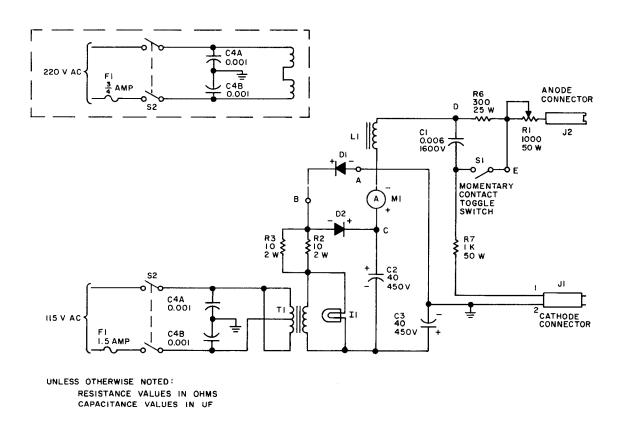
FIGURE 4. SCHEMATIC DIAGRAM OF TYPE 71
